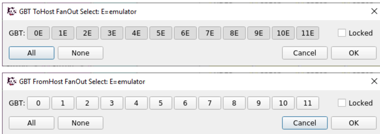
Figure 6.4 Fan out control for to-host (top) and from-host (bottom) directions. The setting for each link is displayed separately (in this case for a 12-link FLX-712 device, i.e. for a 24-link FLX-712 card). It is also possible to (soft)lock the settings using the dedicated checkbox, causing a number of tools to not touch these settings when the lock is set.
